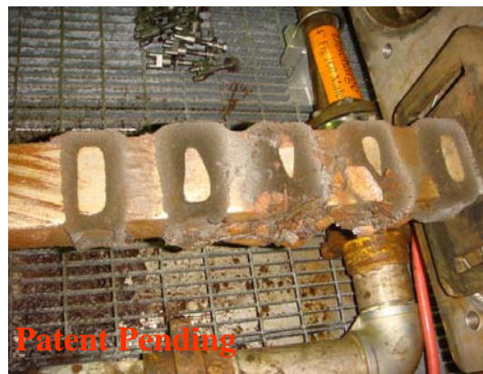
Metal & Iron Oxide from Magnet Cylinders
