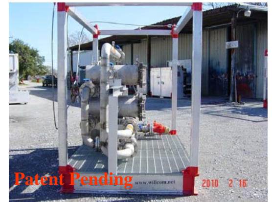
7 - 4" Ball Valves 150# & 1—4" Check Valve MagneTight™ Flow System—Back Left
